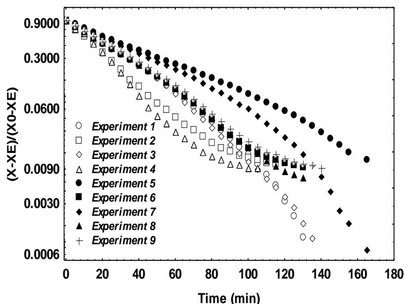
Figure 3 - Curves of the dimensionless free moisture content, in log-linear scale, function of the apple drying time, for the experiments from 1 to 9 of the matrix of the experimental design.
