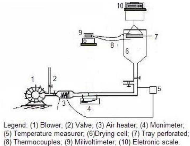
Figure 1 - Scheme of the tray drier with perpendicular air flow.
