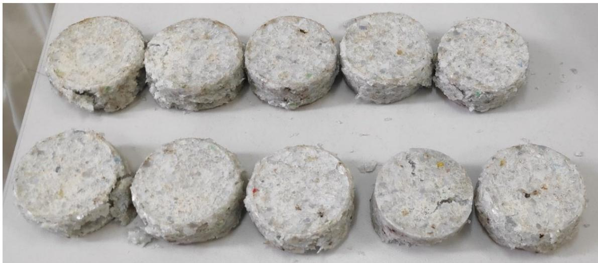
Figure 3: All the ten Specimens after the compression test.
