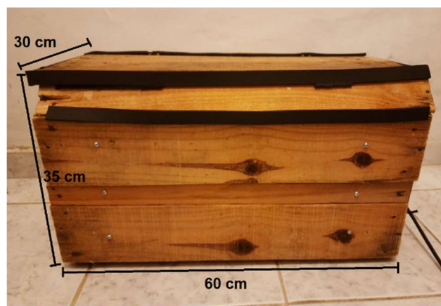
Figure 4: Degradation chamber built in a wooden crate box.
