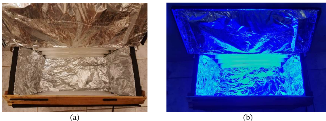
Figure 3: Internal view of the UV chamber, turned off and on.
