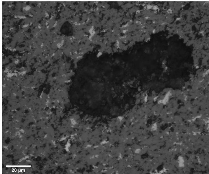
Figure 2: A micropore of 105  $\mu\text{m}$  found in the B<sub>4</sub>C sample with 10% Nb at 500x magnification.
