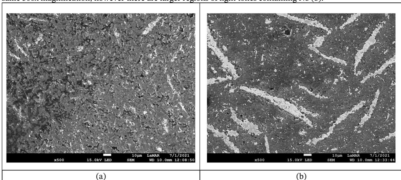
Figure 6: SEM image on B<sub>4</sub>C-Nb composites with 2% Nb (a) and 20% Nb (b) obtained 15 kV.
