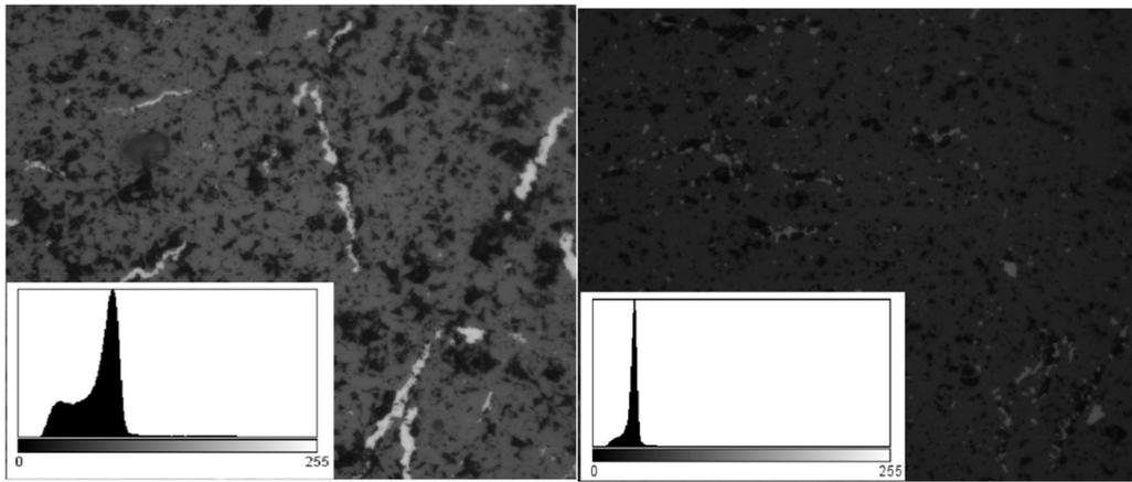
Figure 3: Example of the contrast of the images obtained by MO of the B<sub>4</sub>C samples with 5% Nb and 500x magnification. The histogram (frequency of number of pixels from 0 -1 versus shade of gray from 0 - 255) on the left shows the concentration of hues in the middle part of the scale.
