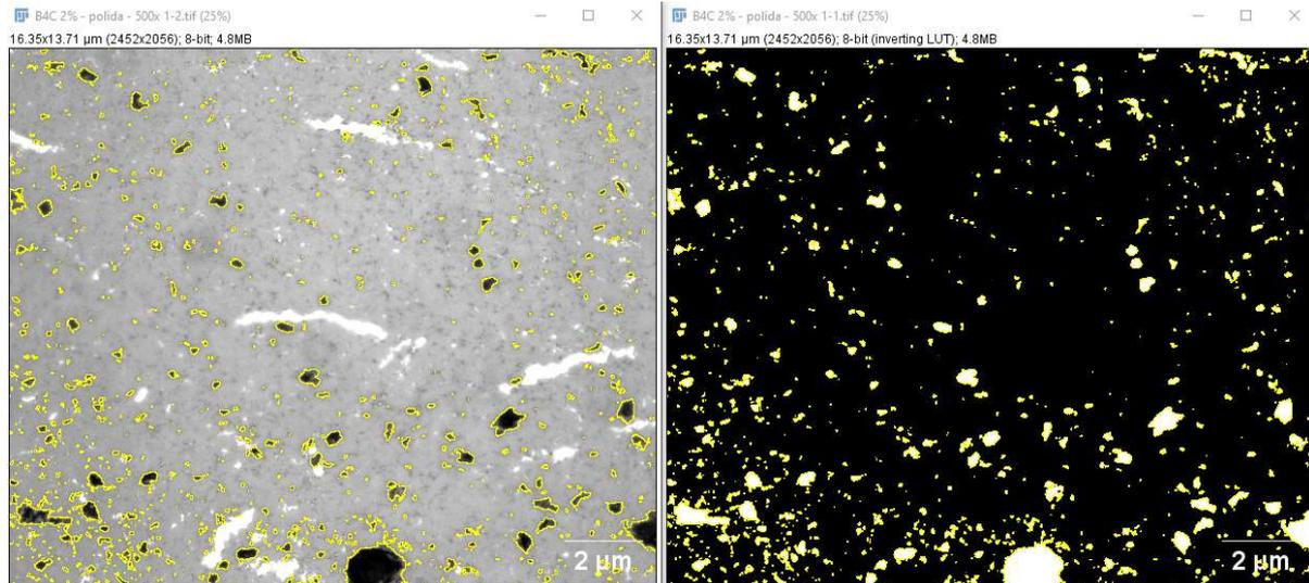
Figure 1: Initial image of the B<sub>4</sub>C-Nb sample with 2% Nb containing pores (dark regions) (a) and the result of the area selected for measurement (white regions) (b).
