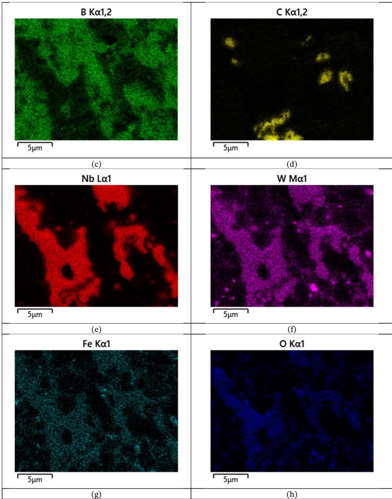
Figure 4: Region of the B<sub>4</sub>C-Nb composite with 20% Nb mapped by EDS (a). B-rich matrix (green) containing Nb-based veins (red) (b). Regions with more intense signal for the chemical elements B (green) (c), C (yellow) (d), Nb (red) (e), W (magenta) (f), Fe (light blue) (g), O (dark blue) (h).
