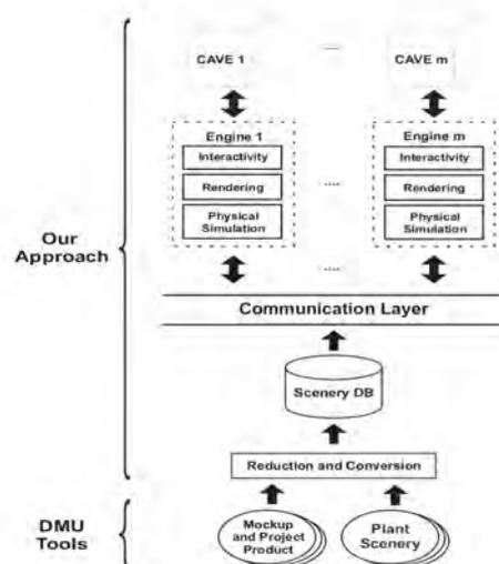
Figure 1: Platform for collaborative visualization of industrial processes
